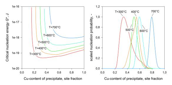
Figure 12 - (a) Critical nucleation energy G\* and the (b) normalized nucleation probability in an Fe-3wt.-%Cu system [49].
