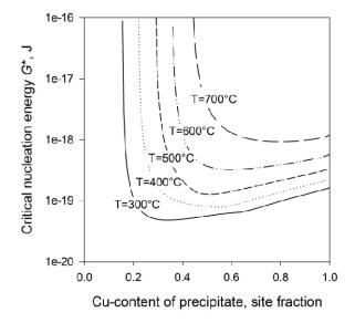
Figure 1 - Calculated nucleation energies as a function of Cu-content from 300 to 700°C.
