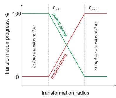
Figure 14 - Schematic reproduction of the radius dependent transformation model applied in this work.
