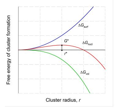
Figure 5 - Free energy of cluster formation as a function of cluster radius.
