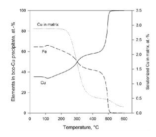
**Figure 4** - Chemical composition of the Cu nucleus as calculated from the minimum  $G^{t}$  concept and its evolution to almost pure Cu at higher temperatures. The dotted curve shows the matrix Cu content.
