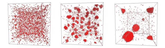
Figure 15 - Monte Carlo calculations of the clustering and coalescence in Fe-3at.-%Cu. Cu is shown in red, matrix Fe is not shown for clarity.
