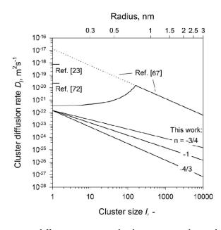
Figure 10 – Cluster and monomer diffusion rates as used in literature together with the classical Binder-Stauffer expression and variation in *n*.
