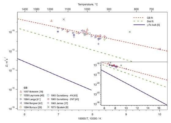
Figure 3 – Experimental data for grain boundary and dislocation pipe diffusion in  $\gamma$ -Fe and corresponding
