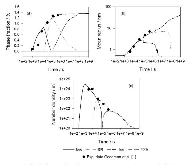
Figure 2 - Results of the kinetic simulation for Fe-1.4 wt.% Cu alloy investigated by Goodman [1]. (a)-(c) show the phase fraction f, mean radius r and number density N of the three considered populations bcc, 9R and fcc. All effects (i) to (v) were considered.
