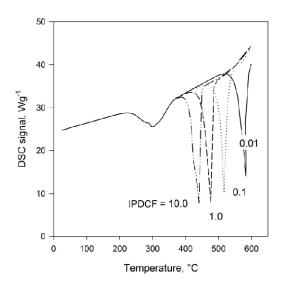
Figure 5 - Simulation of DSC signal with a variation of the inner particle diffusion coefficient factor.
