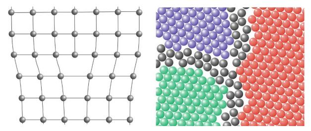
Figure 2 - Schematic reproductions of (left) an edge dislocation and (right) grain boundaries.
