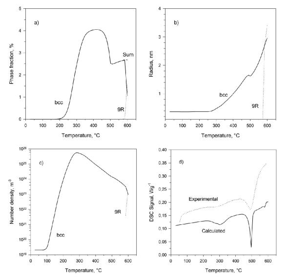
**Figure 2.** Thermokinetic parameter triplet of coherent bcc, semi-coherent 9R and total sum of phases for a) phase fraction, b) radius and c) number density. Calculated and experimental DSC curves are shown in d).
