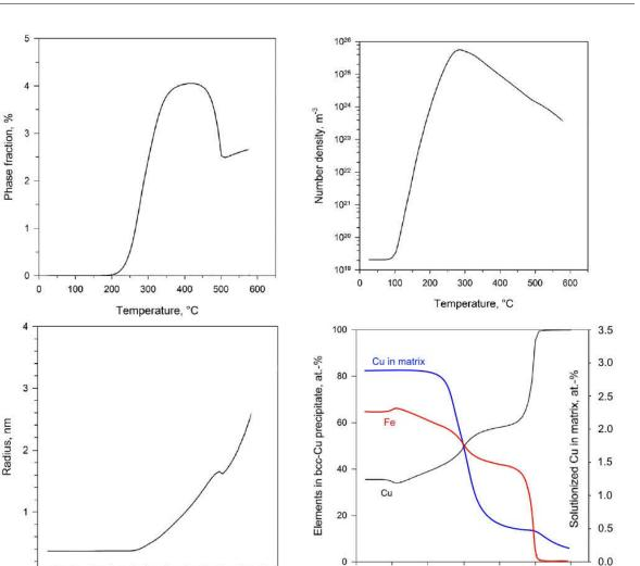
Temperature, °C Figure 16 - Simulation results of 15-5PH steel, showing the thermo-kinetic triplet, phase fraction, number density and radius, together with evolution of chemical composition for precipitate and matrix.
