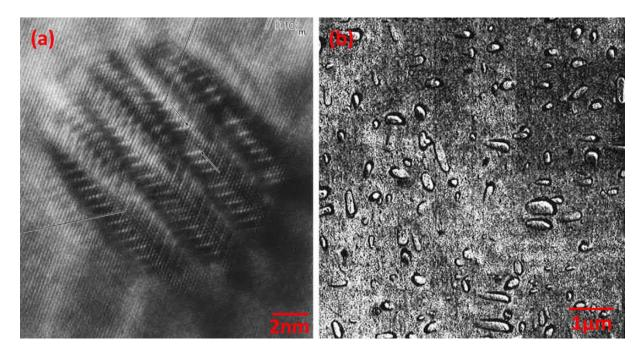
Figure 13 - (a) 9R Cu precipitate in Fe-1.3wt.-%Cu alloy after 100 h annealing at 550 °C, reproduced from ref. [14], reprinted with permission of Taylor & Francis (b) fcc Cu precipitate in Fe-5.4wt.-%Cu alloy after 4 h annealing at 830 °C, reproduced from ref. [15], reprinted with permission of The Minerals, Metals & Materials Society.
