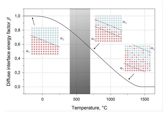
Figure 9 - The diffuse interface energy factor for the regular solution critical temperature of 1750 K as evaluated in the Fe-Cu system. Typical annealing temperature is highlighted by the gray area. Inserts show different states of a sharp interface, being ideally, completely sharp on the very left, to a rather diffuse interface on the right end.
