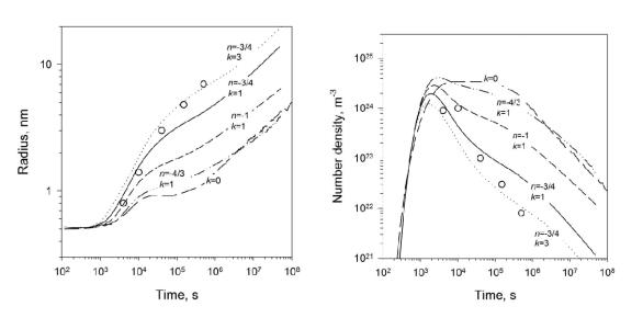
Figure 9 – Evolution of radius and number density with different coalescence factors (*k*) and Binder-Stauffer coefficients (*n*).
