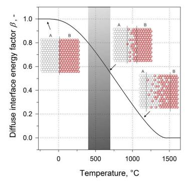
Figure 7 – The diffuse interface energy factor calculated for a regular solution critical temperature of 1750K (1477°C). The temperature region studied in the present report is marked in gray.
