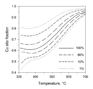
Figure 4 – Normalized nucleation probability as a function of T and  $X_{Cu}$  calculated from the minimum  $\hat{G}$  concept [59].
