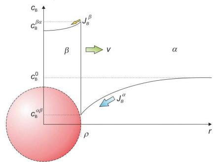
Figure 10 - Schematic representation of a B-rich precipitate growing in a supersaturated matrix.
