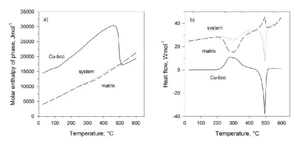
**Figure 3** - a) Molar enthalpy of precipitate phase, ferrite matrix, and the total system, and b) the heat flow of phase, with respect to the actual phase fractions.
