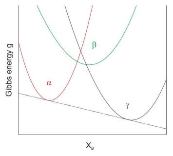
Figure 4 - Gibbs energy curves in a binary A-B alloy. In the present example, the parallel tangent construction delivers a stability region for the  $\alpha$  and  $\gamma$  phases, but no region of  $\beta$  phase stability.
