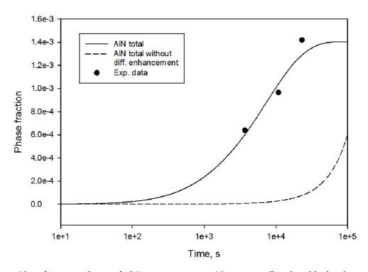
Figure 3 - Phase fraction evolution of AlN in austenite at 1100°C in a microalloyed steel [30] with 0.055 wt.-% Al and 0.024 wt.-% N, determined by analytical chemistry.
