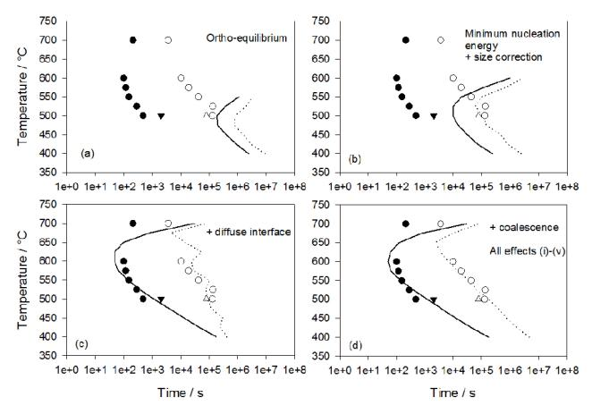
Figure 3 (a)-(d). Calculated ttp-plots for 10% and 90% Cu-precipitation compared with the experimental data referred in [1] triangles and [7] circles, with (a) ortho-equilibrium nucleus composition, (b) minimum G\* nucleus composition and precipitate size effect, (c) entropic effect of mixing at interface and (d) coalescence and, therefore, all different effects (i)-(v).
